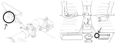
Wheel inflation cover solenoid (located by the exhaust pipe in the motor compartment) is faulty.
